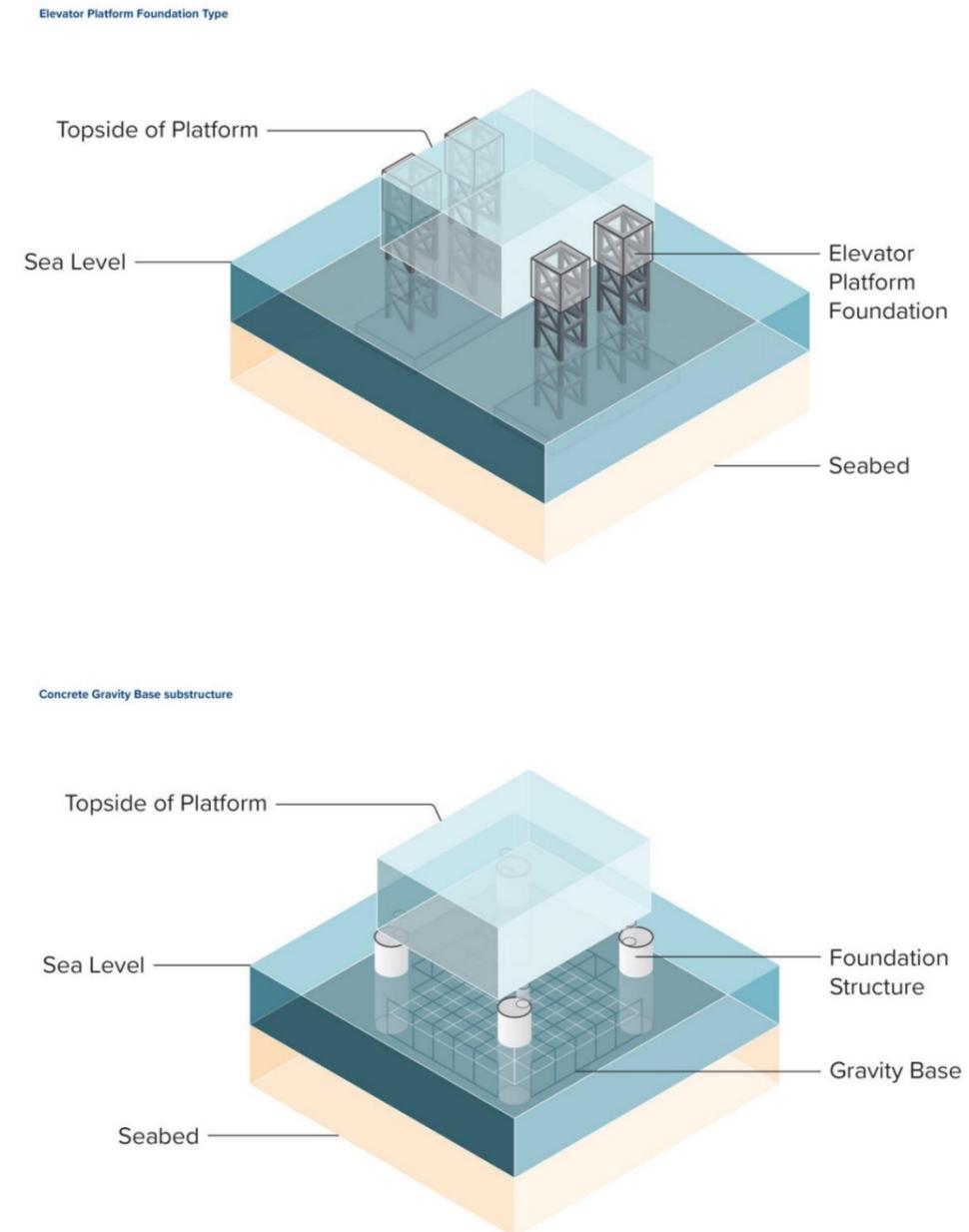
Plate 3-3 Potential Offshore Platform Foundation Types
