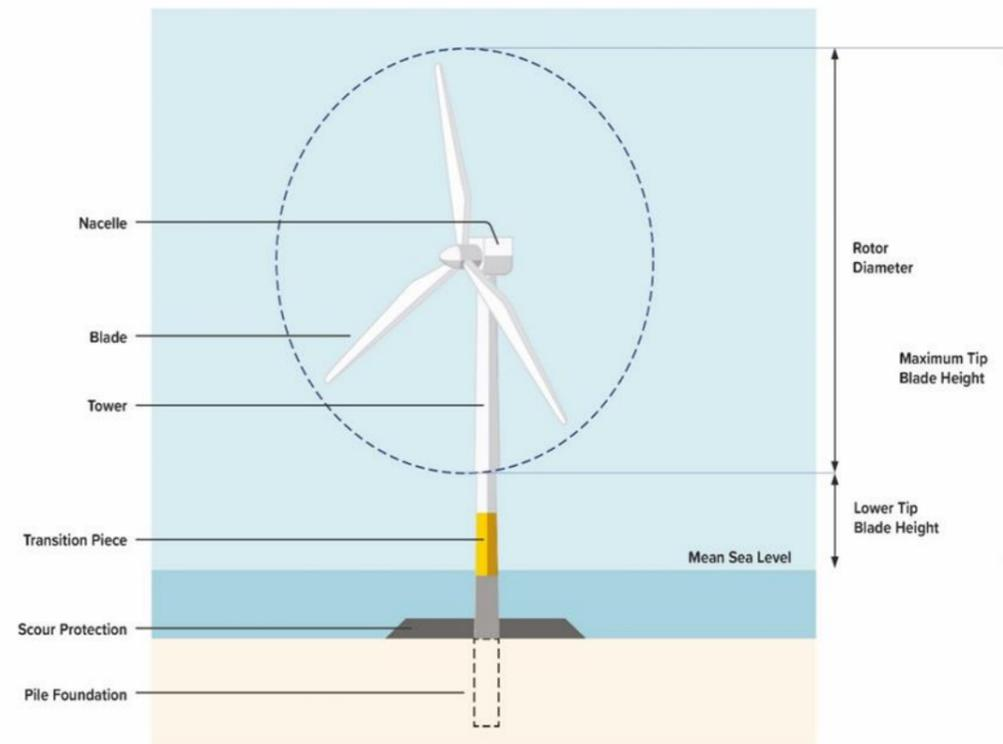
Plate 3-1 Indicative Wind Turbine Schematic
